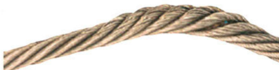
Figure D.4 - Extrusion de torons
